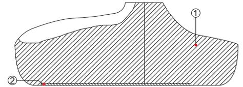
**Structure** Injected flame-retardant foam ① over internal steel frame ② .Base in wood ③.
