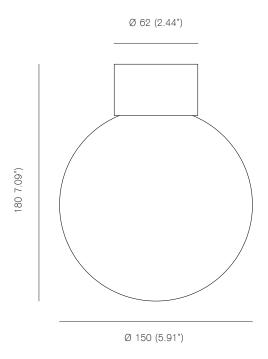
Bulb specifications 240V G9 40W frosted halogen bulb 460 lm / 2800K
