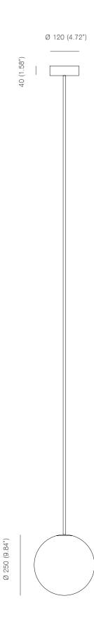
Bulb specifications 240V E14, 40W opal halogen bulb 350lm / 2800K
