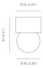
Bulb specifications 120V / 240V G9, 25W frosted halogen bulb 260lm / 3000K
