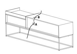
**B** = OPENING FOR CABLE MANAGEMENT Internal dimensions: 65mm x 45mm
