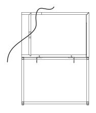
**A** = HOLE FOR CABLE MANAGEMENT Internal dimensions: 60mm x 40mm
