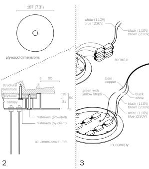
Note: The client is responsible for providing a robust 3/4" (19mm) plywood backing or wood blocking to securely anchor to the structural substrate.
