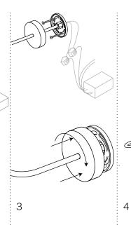
Tuck wiring into wall opening and affix the cover plate with fasteners provided.
