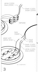
Connect transformers inside the canopy to line voltage, ensuring to match black wire to black wire and white to white. For the ground connection, connect the green wire with yellow stripe to the bare copper wire or green wire in the junction box.
