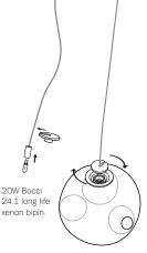
Each pendant terminates in a "headphone jack" type connector, which plugs into a receiving receptacle in the canopy. After plugging in each pendant, turn the threaded sheathing into place by hand ensuring that it is adequately tightened. Tools are not required.
