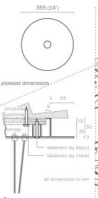
Note: The client is responsible for providing a robust 3/4" (19mm) plywood backing or wood blocking to securely anchor to the structural substrate.
