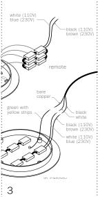
Connect transformers inside the canopy to line voltage, ensuring to match black wire to black wire and white to white. For the ground connection, connect the green wire with yellow stripe to the bare copper wire or green wire in the junction box.
