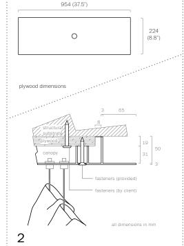
Note: The client is responsible for providing a robust 3/4" (19mm) plywood backing or wood blocking to securely anchor to the structural substrate.
