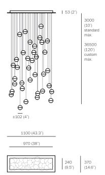
The 14 is an articulated, seamed cast glass sphere with a frosted cylindrical void that houses either a low voltage (12V, 10W halogen/xenon) or LED(12V, 1.5W) lamp. Individual pendants are visually quite subtle, but gain tremendous strength when multiplied and clustered in large groups.
