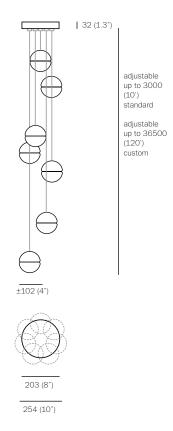
The 14 is an articulated, seamed cast glass sphere with a frosted cylindrical void that houses either a low voltage (12V, 10W xenon) or LED(12V, 1.5W) lamp. Individual pendants are visually quite subtle, but gain tremendous strength when multiplied and clustered in large groups.
