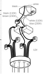
Xenon/Halogen/LED: Connect the coaxial cable to the open slots in the terminal block on the 12V side of the transformers. Ensure that the braided outer wires are all connected to one 12V output wire and all inner insulated wires are connected to the other or a short will occur.
