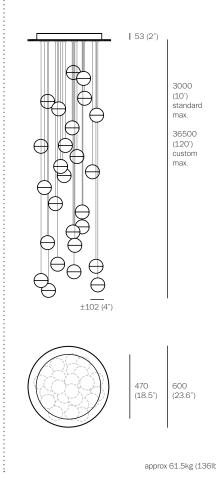
The 14 is an articulated, seamed cast glass sphere with a frosted cylindrical void that houses either a low voltage (12V, 10W halogen/xenon) or LED(12V, 1.5W) lamp. Individual pendants are visually quite subtle, but gain tremendous strength when multiplied and clustered in large groups.
