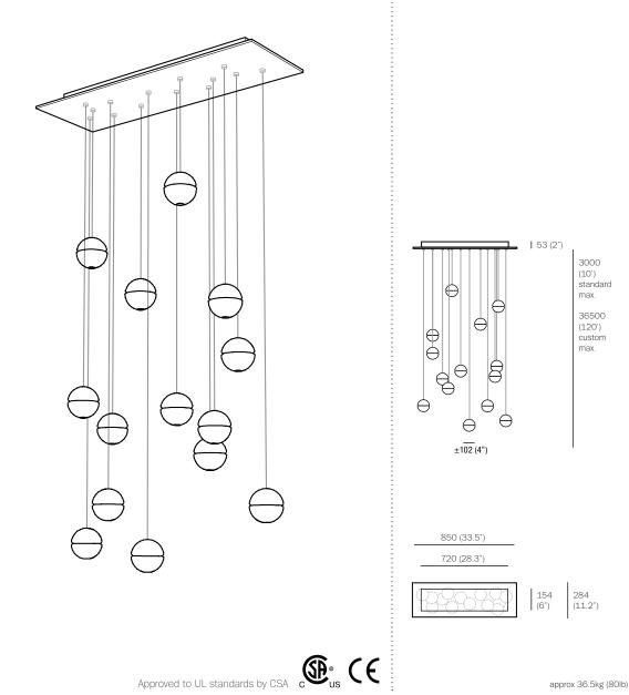
The 14 is an articulated, seamed cast glass sphere with a frosted cylindrical void that houses either a low voltage (12V, 10W halogen/xenon) or LED(12V, 1.5W) lamp. Individual pendants are visually quite subtle, but gain tremendous strength when multiplied and clustered in large groups.
