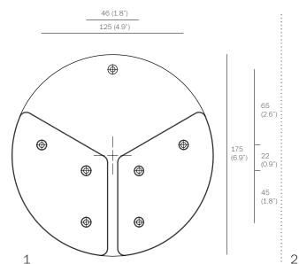
Locate centre point location on wall where the 19 will be mounted and use the wall cleat or the above diagram to mark the screw holes.
